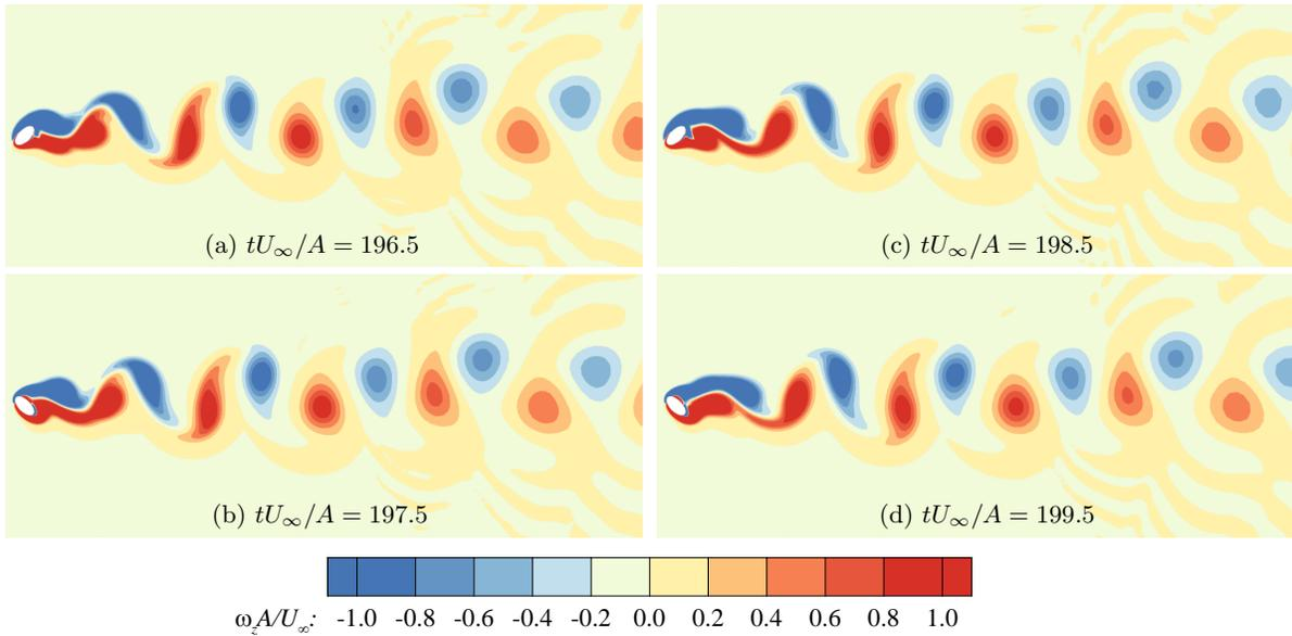
Figure 24. Vorticity contours for flow over a rotating elliptic cylinder using a rigid-rotating mesh.
