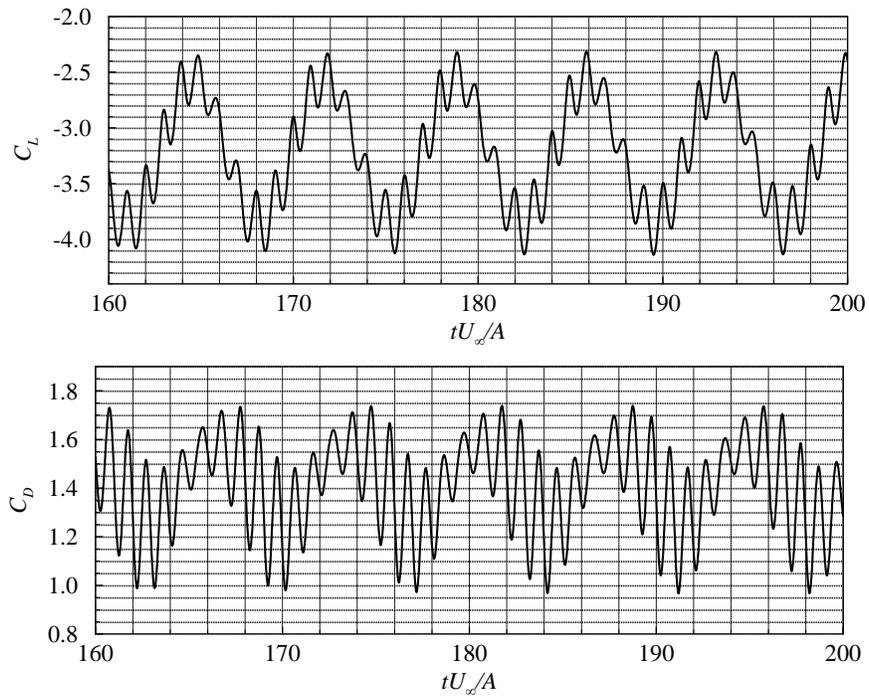
Figure 31. Converged lift and drag coefficients for flow over a rotating square cylinder.
