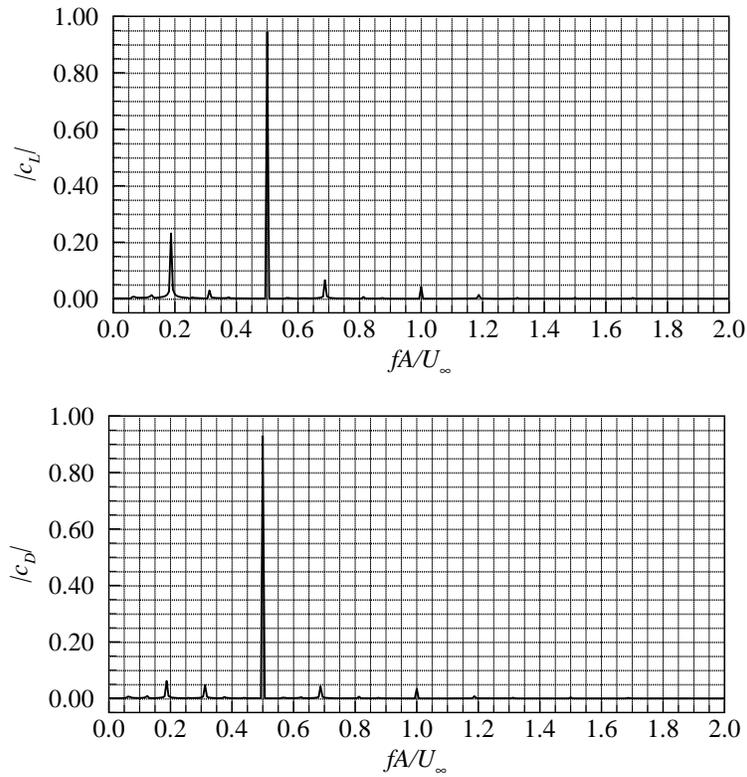
Figure 22. Spectrum of unsteady lift and drag coefficients for flow over a rotating elliptic cylinder.
