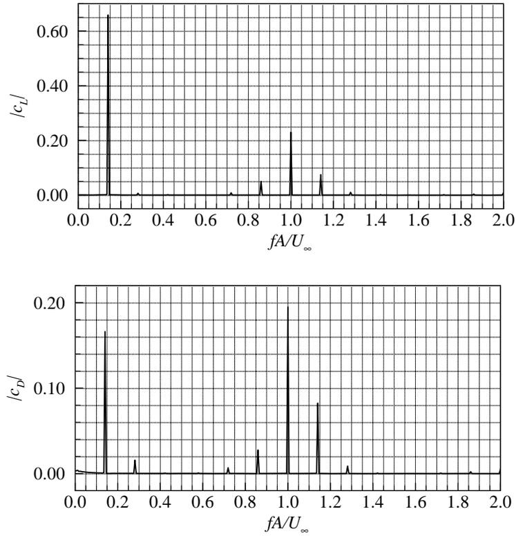
Figure 33. Spectrum of unsteady lift and drag coefficients for flow over a rotating square cylinder.
