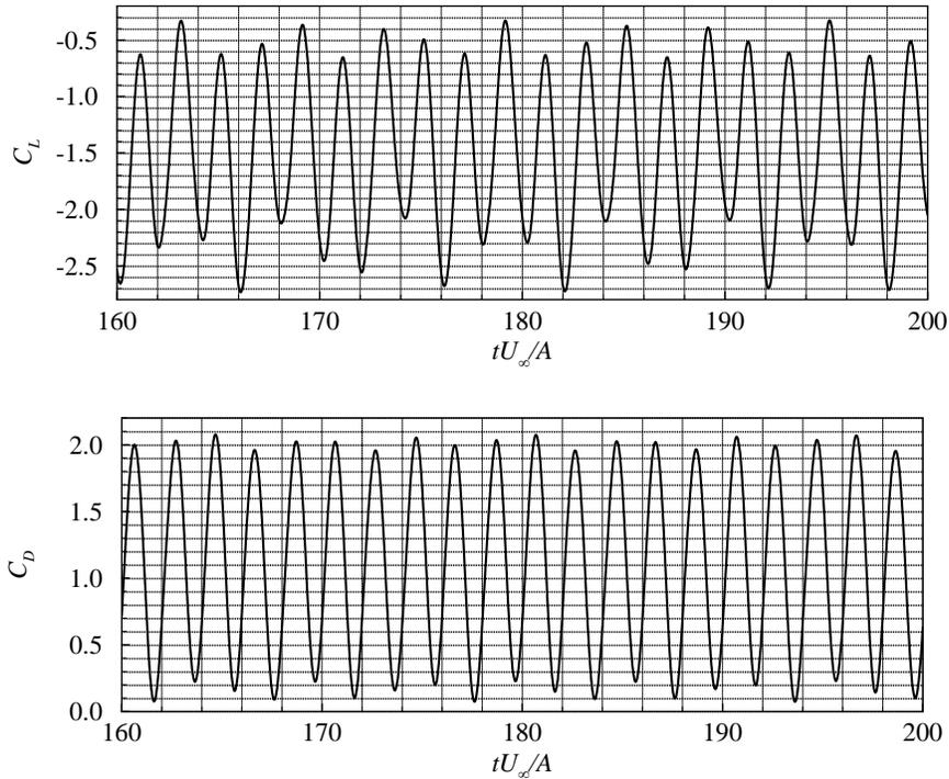
Figure 20. Converged lift and drag coefficients for flow over a rotating elliptic cylinder.
