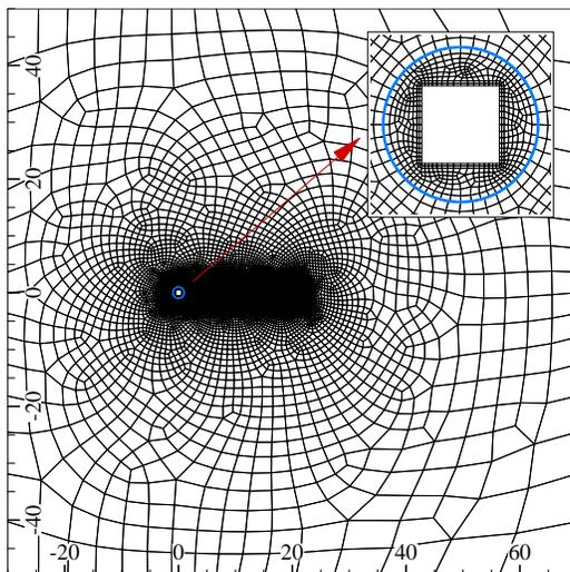
Figure 30. Mesh for a rotating square cylinder (blue circle indicates sliding interface).
