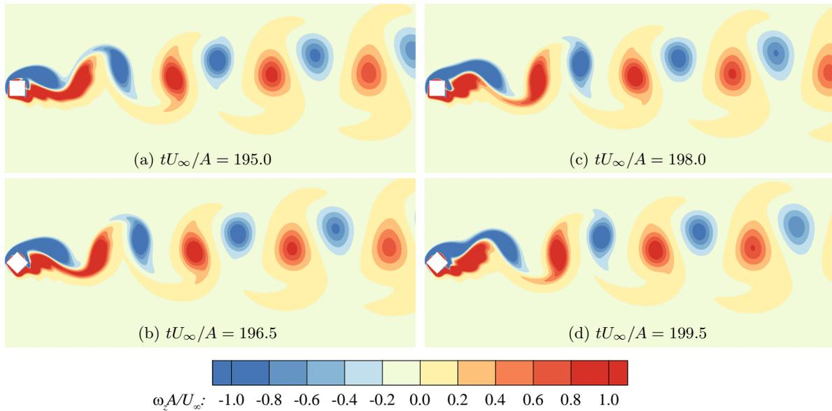
Figure 34. Vorticity contours for flow over a rotating square cylinder.
