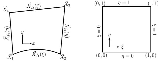
**Figure 3.** Transfinite mapping of a physical element to a standard square element.
