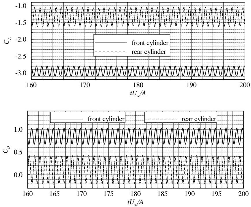
Figure 36. Converged lift and drag coefficients of two tandem rotating square cylinder.
