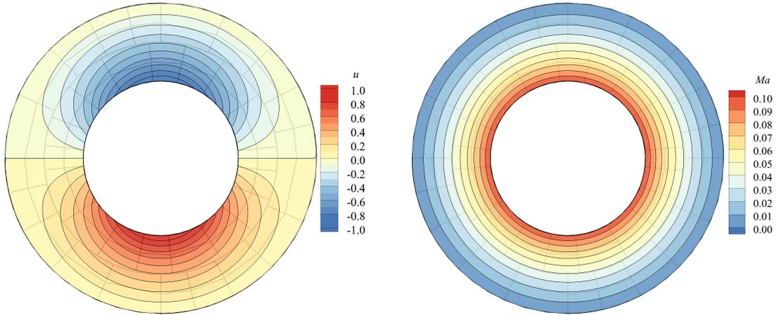
Figure 10. Steady state contours of the Taylor-Couette flow from the 4<sup>th</sup>-order scheme.
