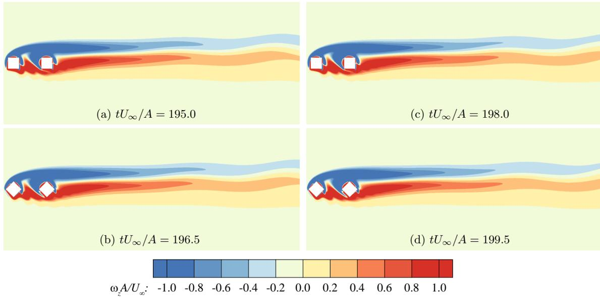
Figure 39. Vorticity contours for flow over two tandem rotating square cylinders.
