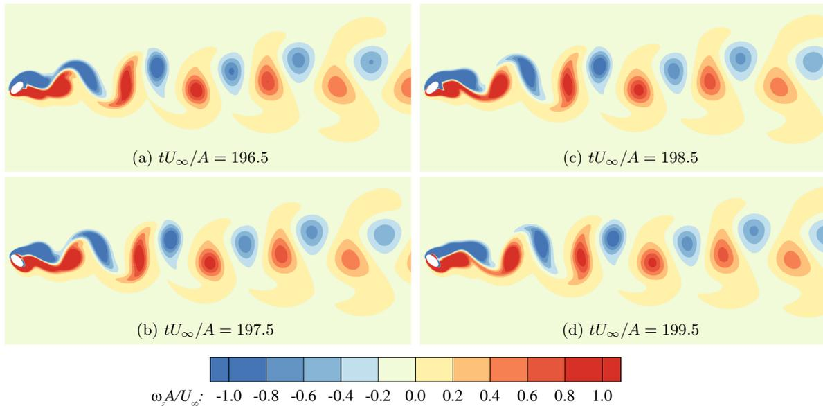
Figure 23. Vorticity contours for flow over a rotating elliptic cylinder using a sliding mesh.
