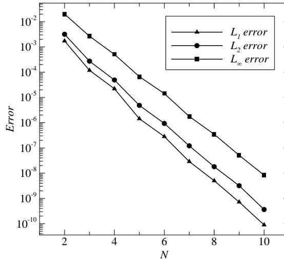
Figure 9. Errors against scheme order on the Euler-vortex flow.
