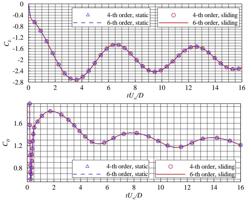
Figure 13. Comparison of transient lift and drag coefficients for a rotating circular cylinder from the 4-th and the 6-th order schemes on a static and a sliding meshes.
