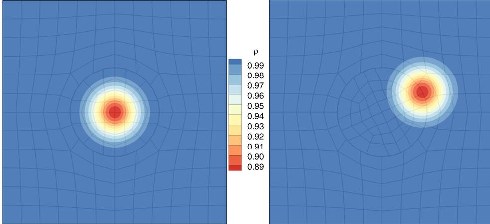
Figure 8. Density contours of the Euler-vortex flow at  $t = 0$  (left) and  $t = 2$  (right) from the 4<sup>th</sup>-order scheme.
