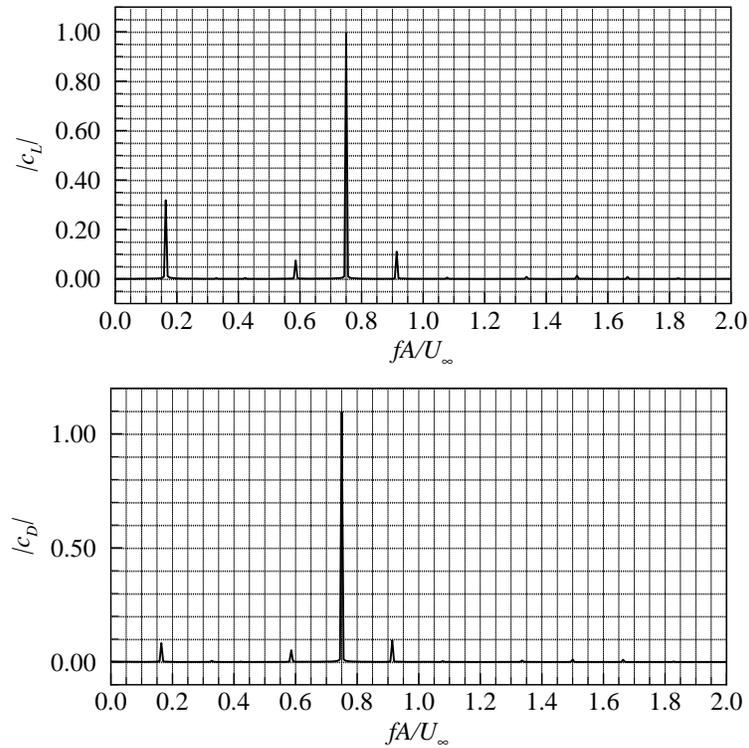
Figure 28. Spectrum of unsteady lift and drag coefficients for flow over a rotating triangular cylinder.
