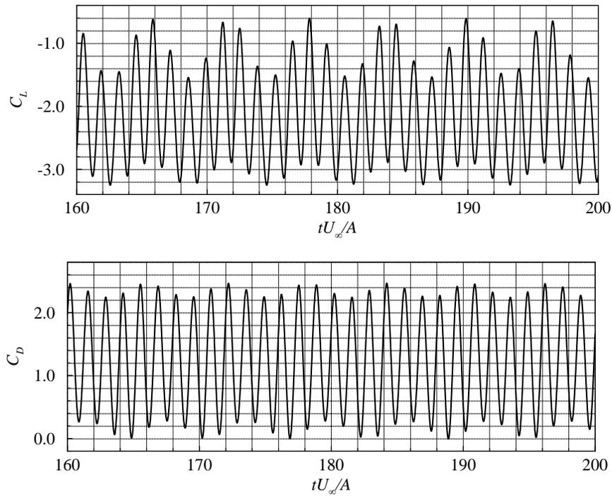
Figure 26. Converged lift and drag coefficients for flow over a rotating triangular cylinder.
