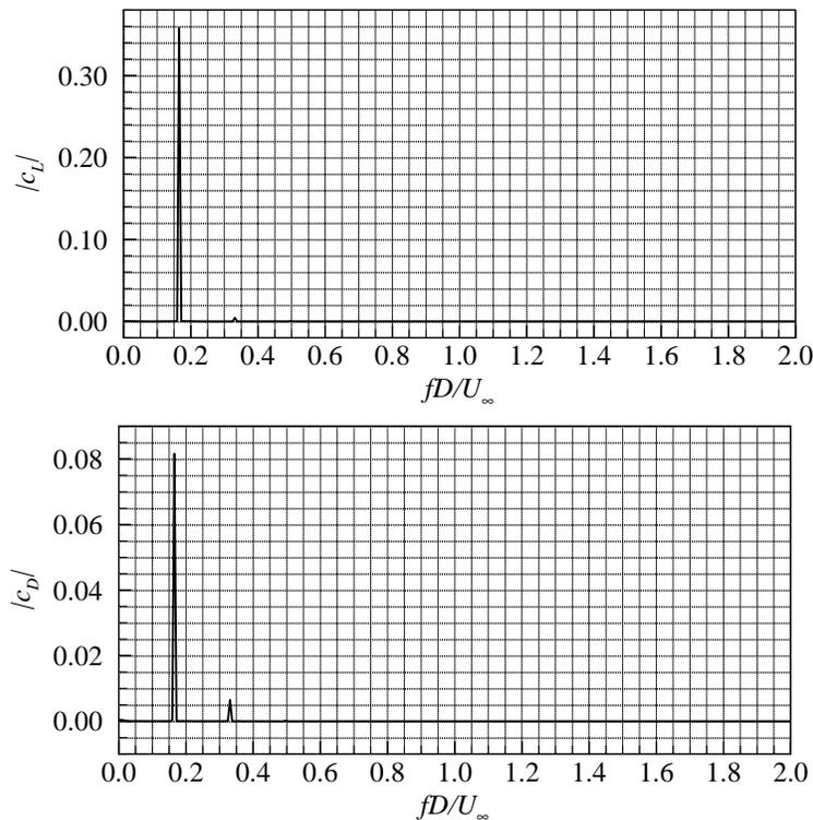
Figure 16. Spectrum of unsteady lift and drag coefficients for flow over a rotating circular cylinder.
