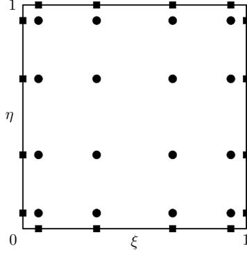
**Figure 4. Schematic of the distribution of solution points (circular dots) and flux points (square dots) for a fourth-order FR scheme.**
