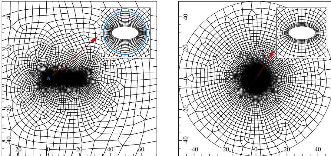
Figure 18. Global and local views of the sliding mesh (blue circle represents sliding interface) and the rigid-rotating mesh (right) for a rotating elliptic cylinder.
