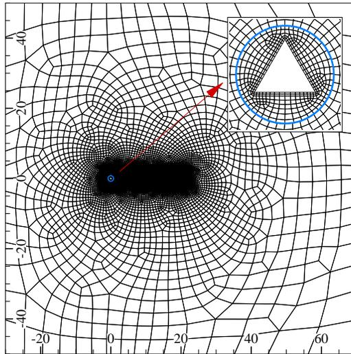
Figure 25. Mesh for a rotating triangular cylinder (blue circle indicates sliding interface).
