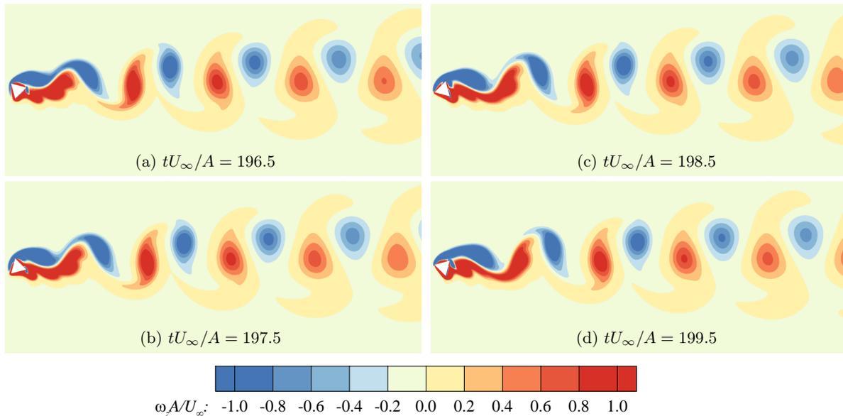
Figure 29. Vorticity contours for flow over a rotating triangular cylinder.
