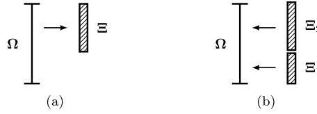
Fig. 4. Projection between face and mortar: (a) from left face to left side of mortar, (b) from two mortars back to the associated left face.
