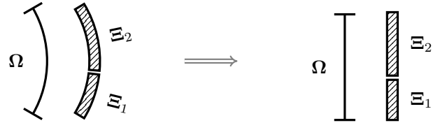
FIGURE 3. Mapping of curved cell face and mortars to straight ones: left, curved face and mortars in physical domain; right, straight face and mortars in computational domain.
